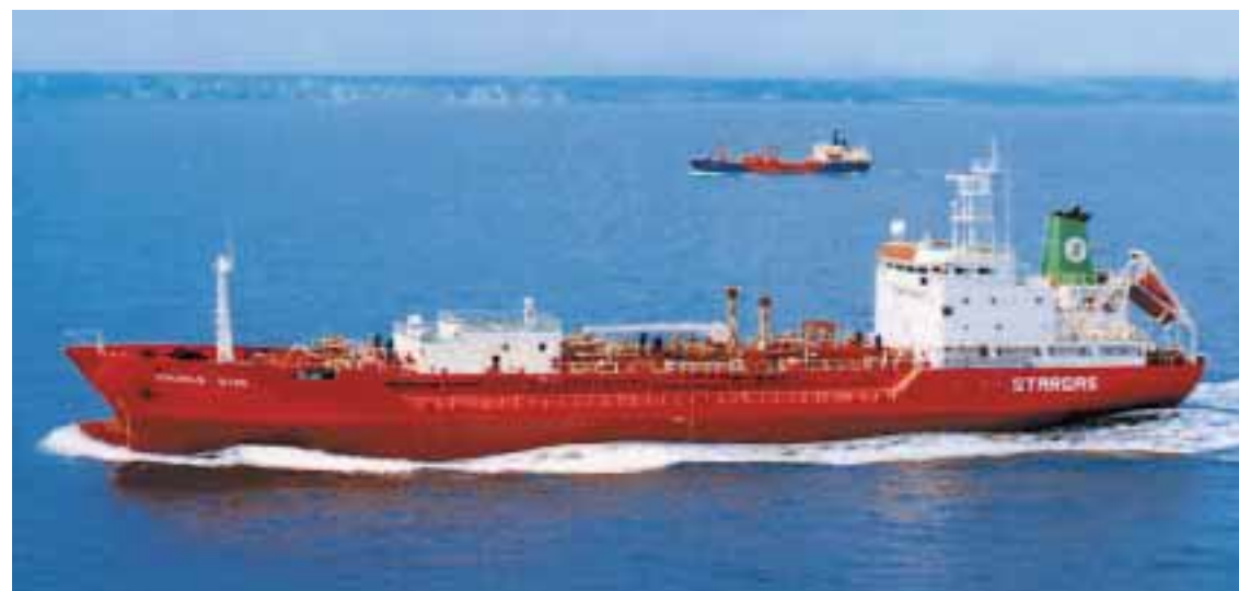
Emerald Star 7,464 cbm ethylene carrier, blt 1992 by I.N.M.A., owned by Stargas and operated by the Gaschem-Medgas pool
