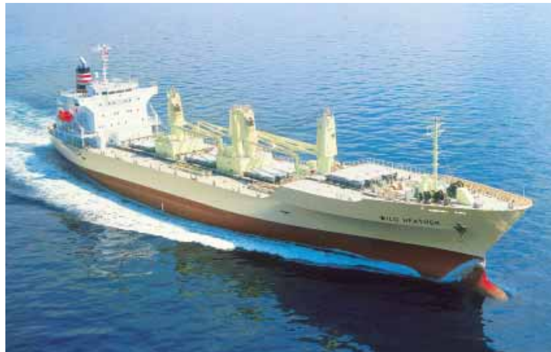
Wild Heather 499,793 cu ft, 58 feus, 58 plugs, 20 kn, 10,144 dwt, blt in 1998 by Iwagi Zosen, operated by NYK-Star Reefers
