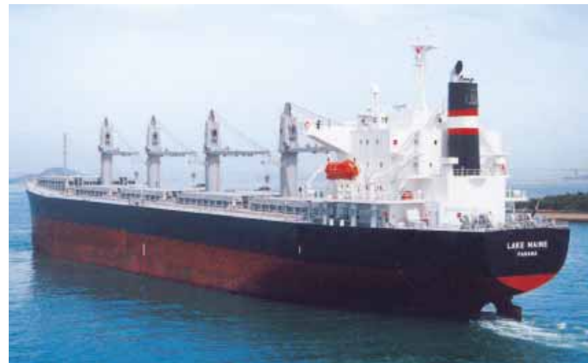
Lake Maine 53,500 dwt, grab-fitted blt 2001 by Imabari Shipbuilding, owned by Daio Kaiun Ltd (Japan) and on long time charter to Louis Dreyfus Armateurs (France)
