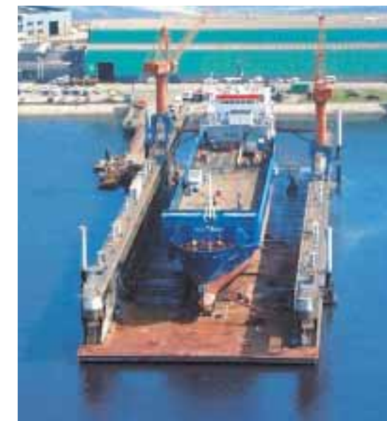
Floating dock 16,000 t lifting capacity, sold by Flender Werft to Dunkirk Port Authority
